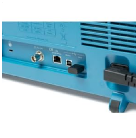
Figure 5.1: Close-up view of the rear panel connectivity ports.
