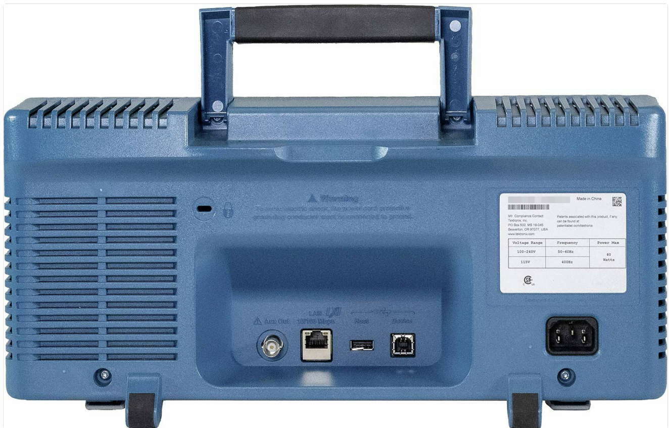
Figure 3.1: Rear panel of the oscilloscope with power input and connectivity ports.
