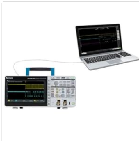
Figure 5.2: The oscilloscope connected to a laptop for data transfer or remote control.
