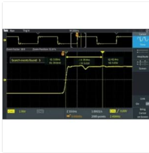
Figure 4.4: Waveform display demonstrating the search and mark function.
