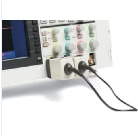
Figure 4.2: Connecting probes to the oscilloscope input channels.
