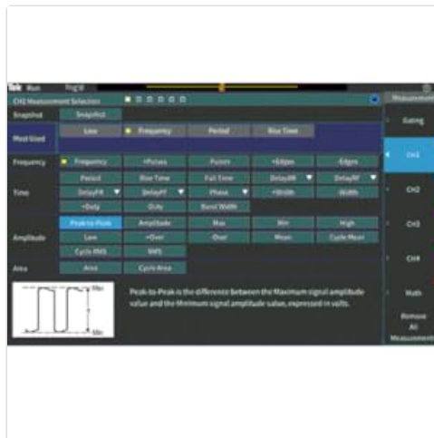
Figure 4.3: The automatic measurement selection menu on the oscilloscope display.
