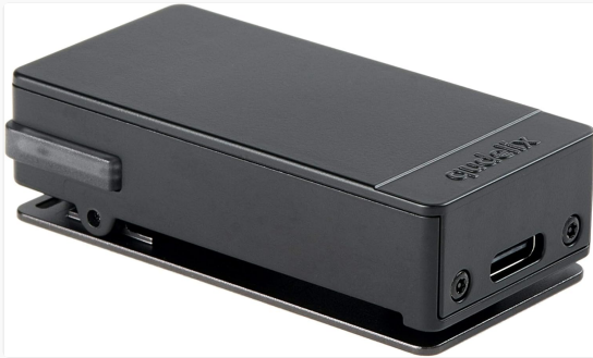
Side view of the Qudelix-5K, showing the USB-C port for charging and data connection.
