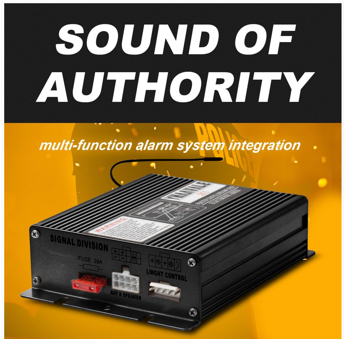
Figure 4.1: Close-up view of the YHAAVALE X5UB amplifier unit, showing the fuse (20A) and connection ports for battery, speaker, and light control.
