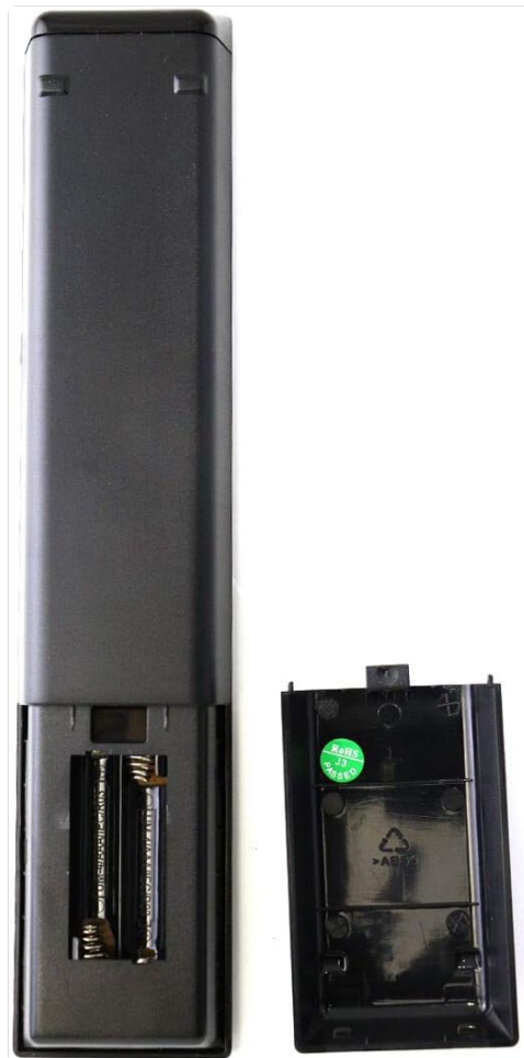
Figure 2: Back view of the XVEFAT remote control, showing the open battery compartment for AAA batteries.
