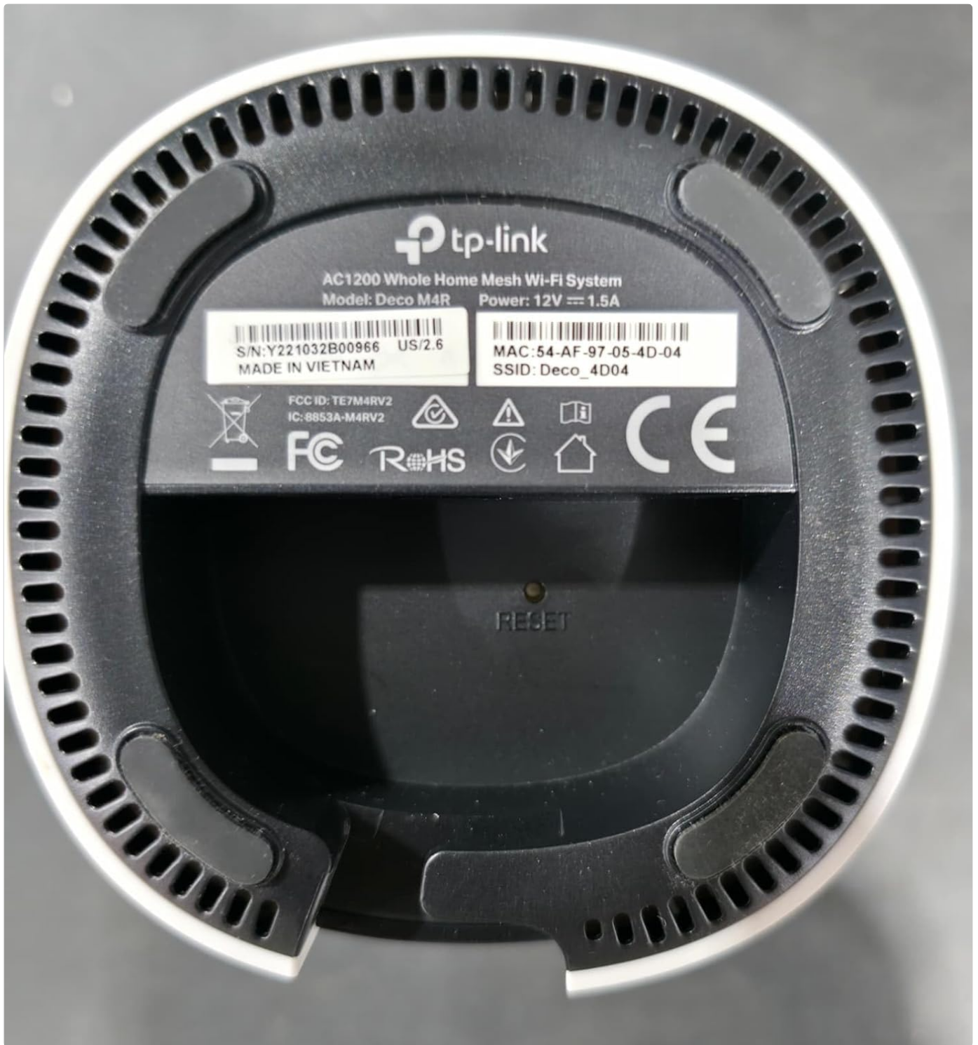
Image: The underside of a Deco M4 unit, displaying important identification details such as model number (AC1200), serial number, MAC address, and the location of the reset button.
