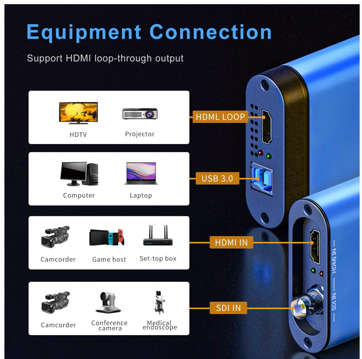
Image: A diagram illustrating the various connection points on the UNISHEEN UC3300HS capture card, including HDMI IN, SDI IN, USB 3.0, and HDMI LOOP, and their respective connections to source devices and displays.
