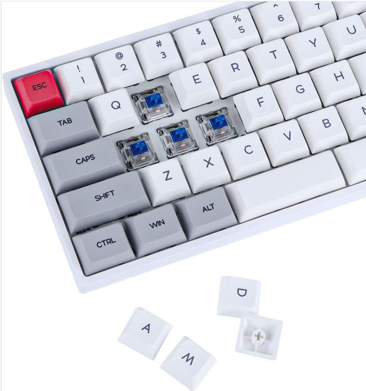
Image: A close-up view of the EPOMAKER SK66 keyboard, showing removed keycaps and exposed Gateron Optical switches, along with loose keycaps.
