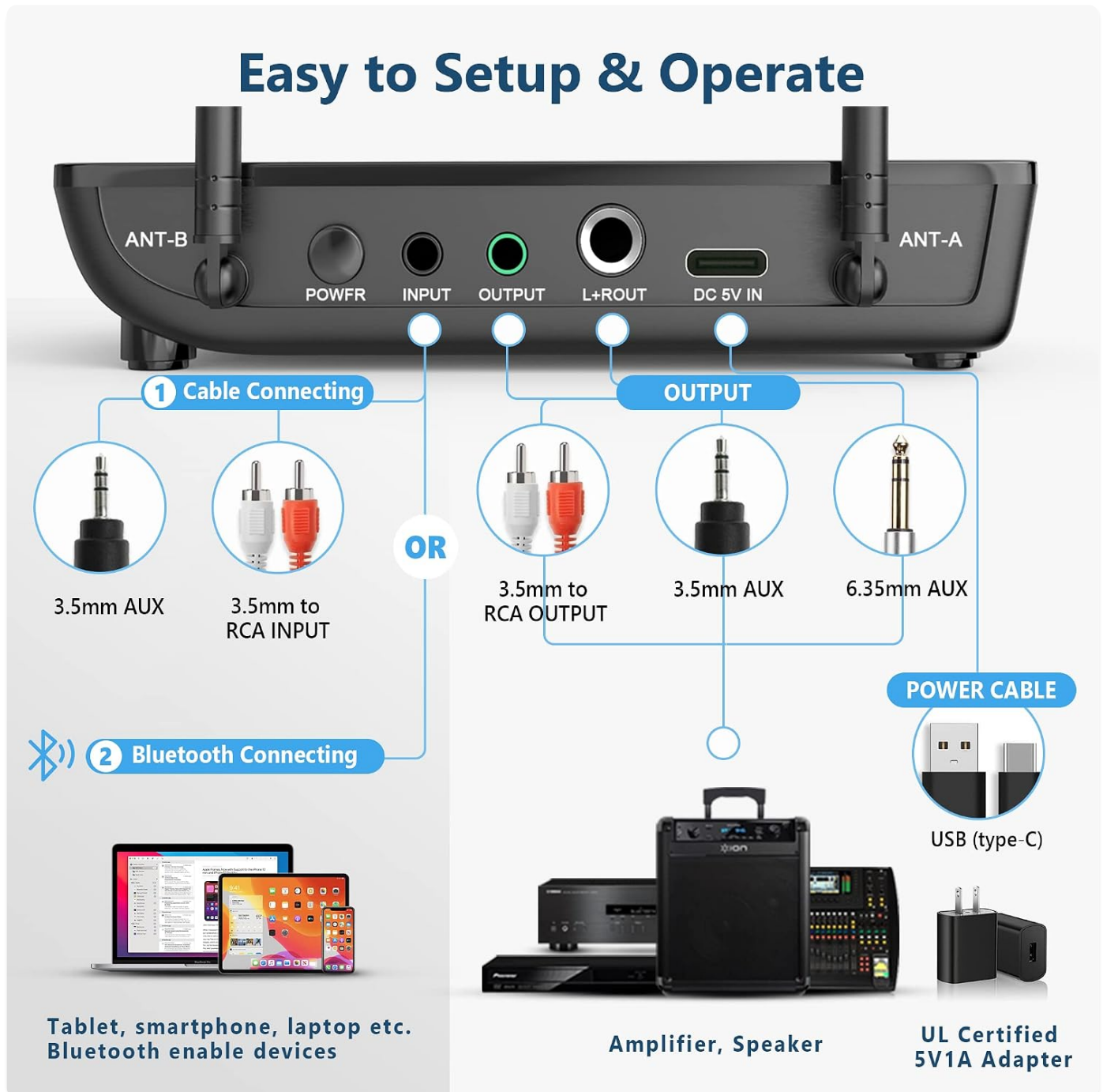
Image: Detailed diagram showing how to connect the receiver to amplifiers, speakers, and other devices using various audio cables.
