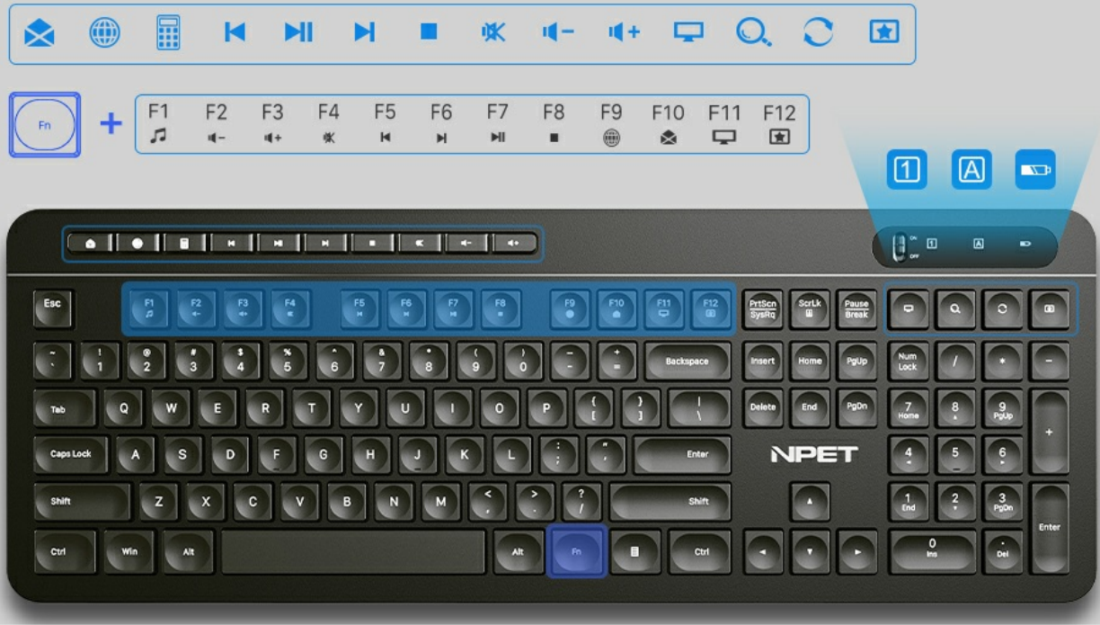
Figure 8: Detailed illustration of hotkey functions and Fn key combinations for improved working efficiency.
