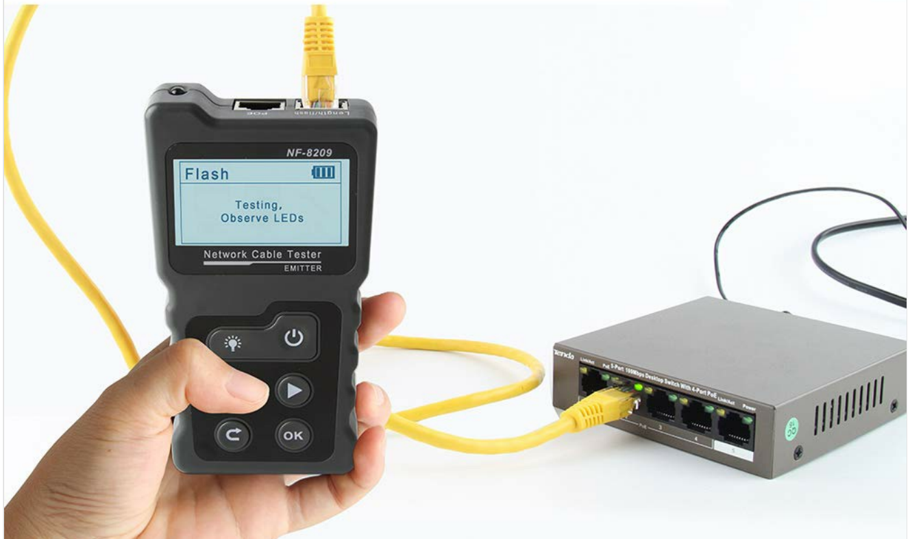
Image: The NF-8209 Emitter connected to a network switch, demonstrating the port flash function to identify the connected port.
