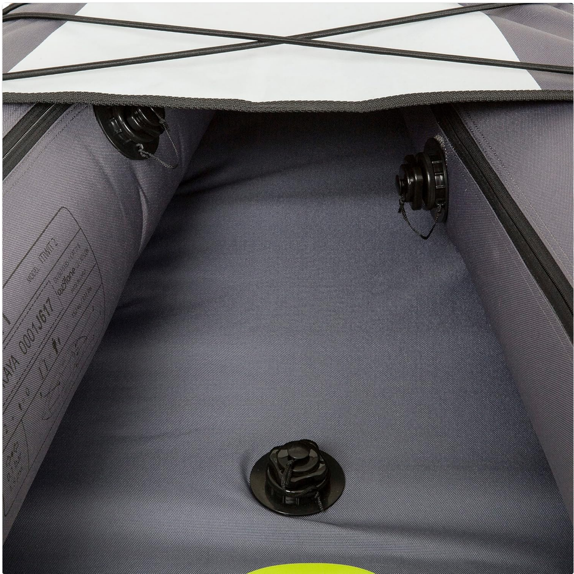
Image 2.1: Detail of the inflation valves on the kayak, showing the secure cap design.
