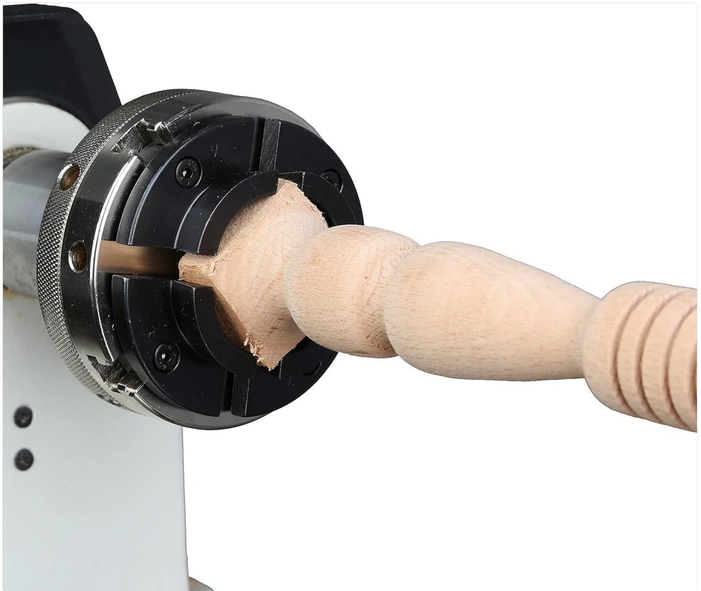
Figure 4.2: The chuck securely holding a workpiece during a turning operation.
