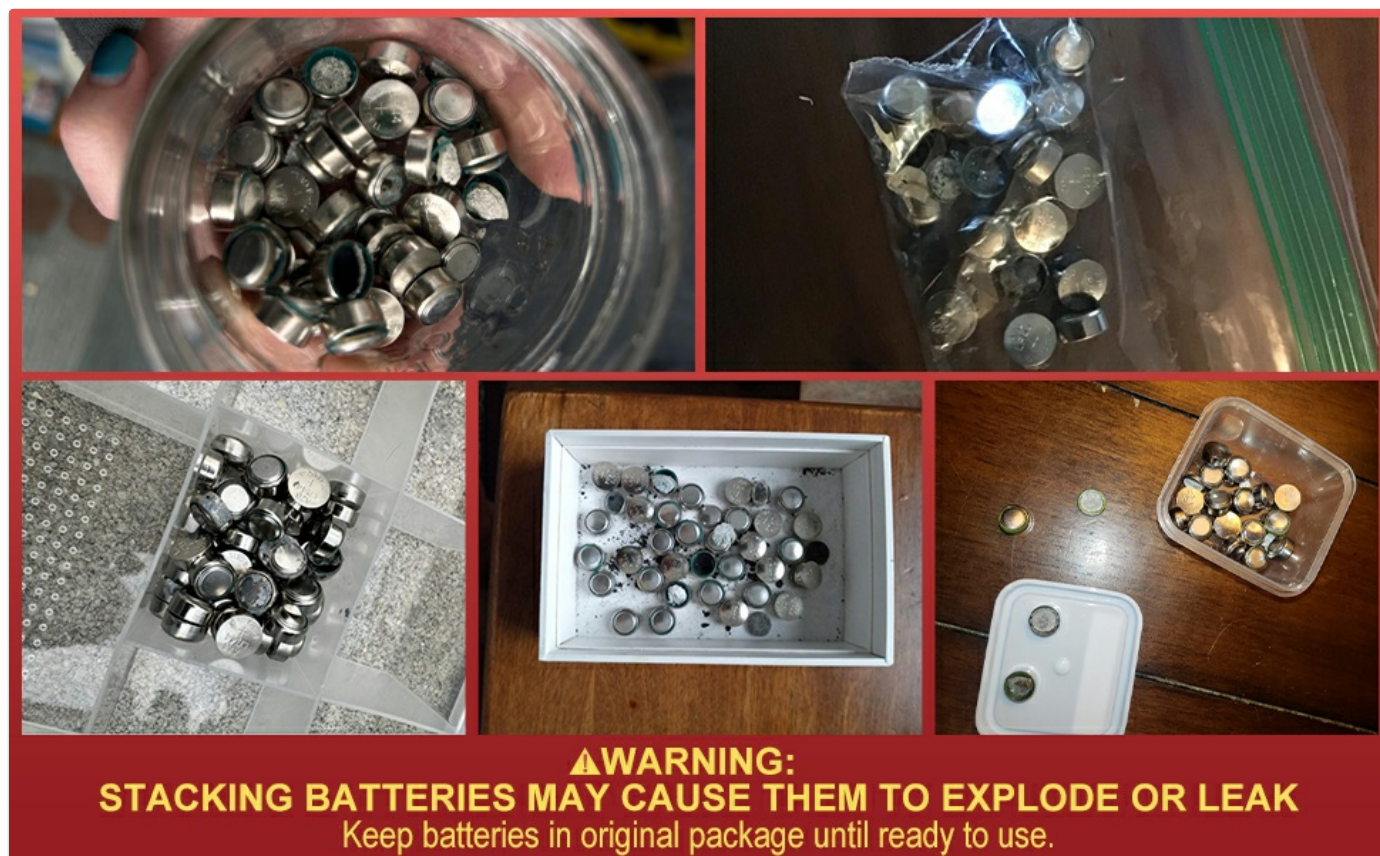
Figure 4: Examples of improper battery storage, which can lead to leakage or explosion.
