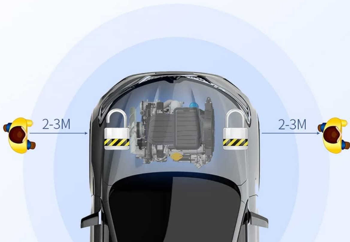
Figure 3: Diagram illustrating automatic engine lock and unlock based on remote proximity (2-3 meters).
