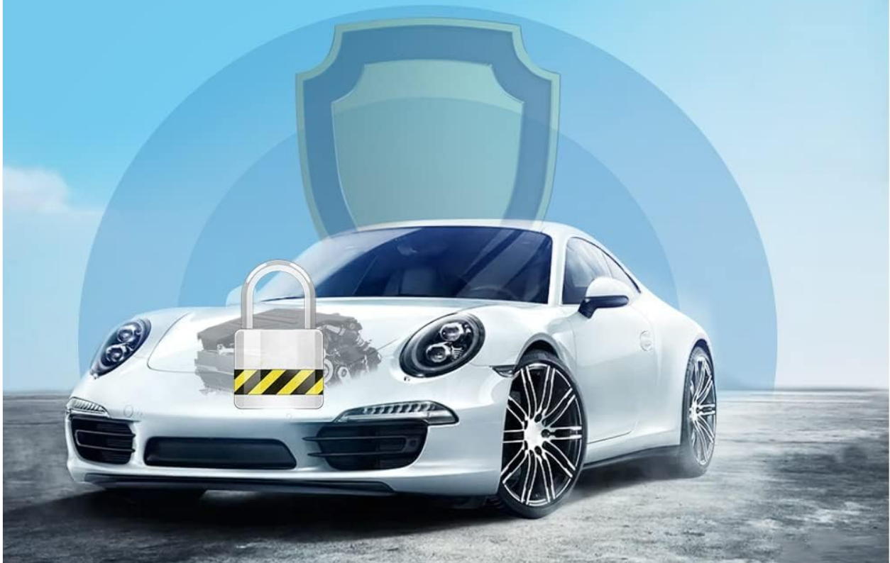
Figure 6: Anti-Hijacking Feature. This graphic depicts a car with a locked engine icon, illustrating the anti-hijacking mode which activates if the remote signal is not detected while the ignition is on, leading to engine shutdown after 70 seconds.
