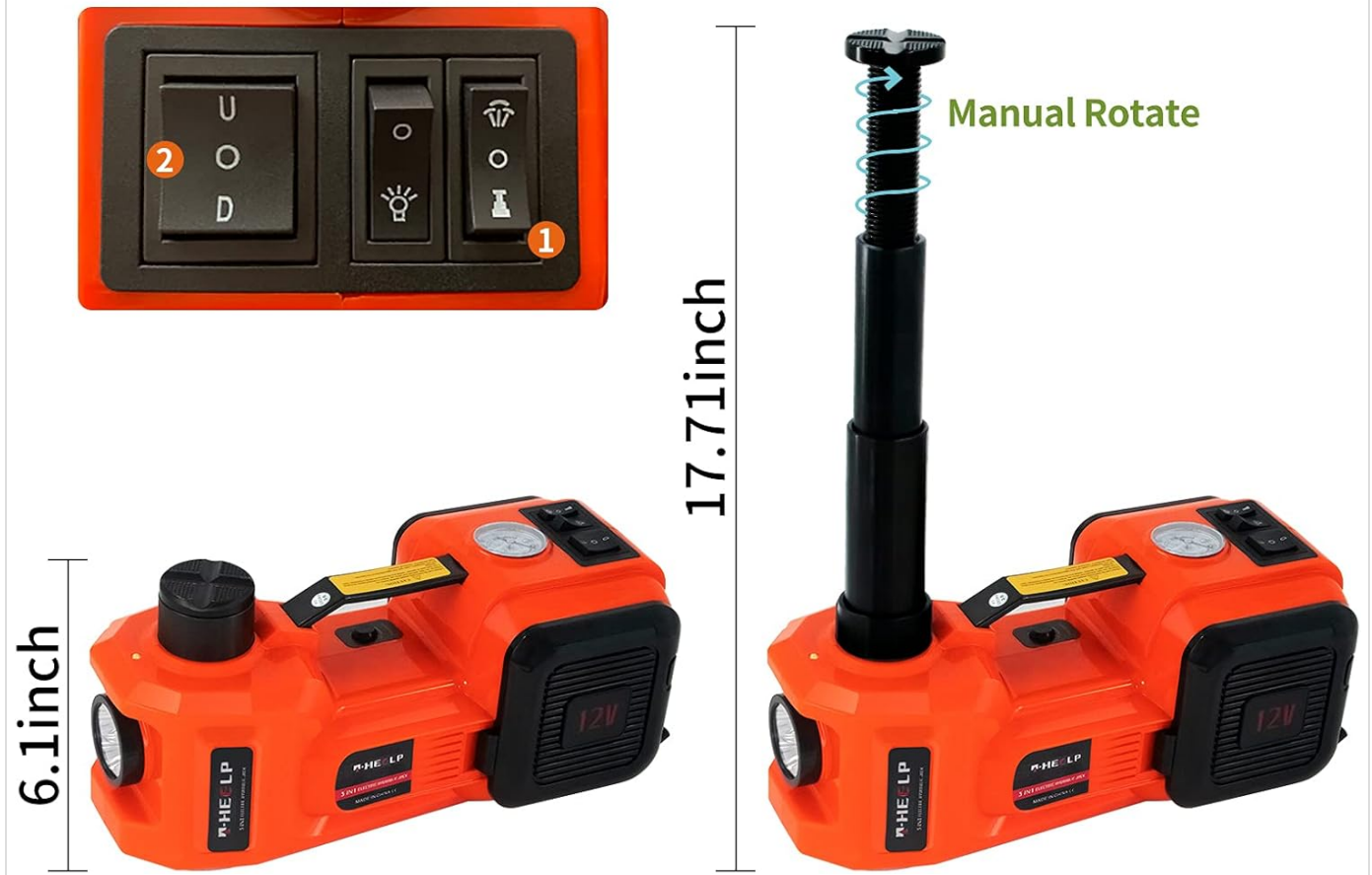
Image: The electric jack is shown in its retracted state (6.1 inches) and extended state (17.7 inches), with an arrow indicating the manual rotation of the plunger for initial height adjustment.
