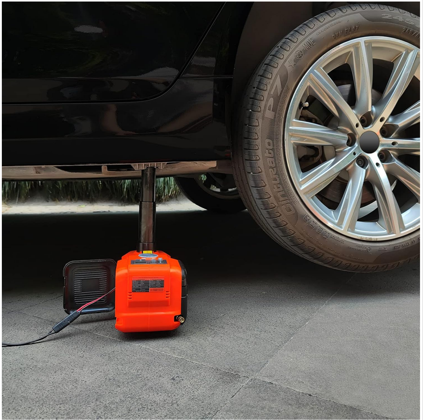
Image: A side view of the electric hydraulic jack lifting a vehicle, demonstrating the clearance achieved for tire changes or maintenance.
