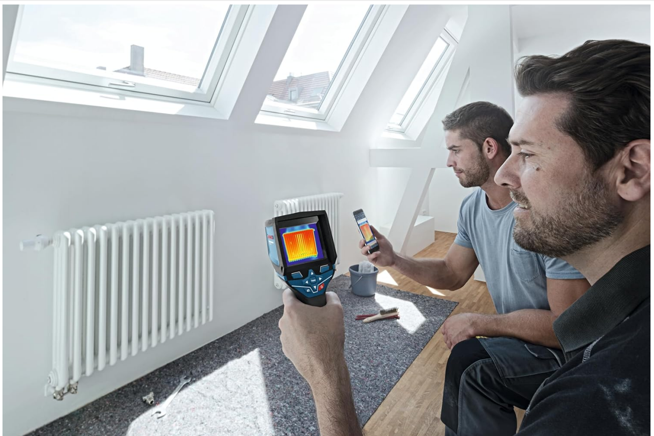
Figure 5.4: Thermal inspection of a radiator. This image shows the GTC400C being used to analyze the heat distribution of a radiator, which can help identify inefficient areas or blockages.
