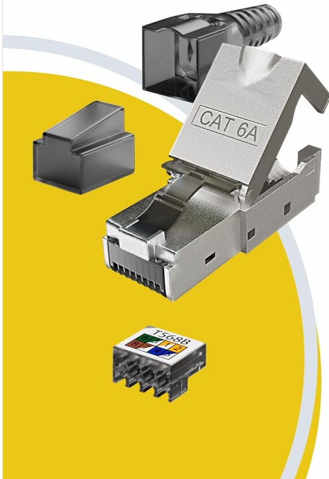
Figure 6: The cable manager component of the RJ45 connector. This image highlights its role in easy, tool-free installation with T568-A/B assignment, reusability, and compatibility with cable diameters of 6-8 mm.
