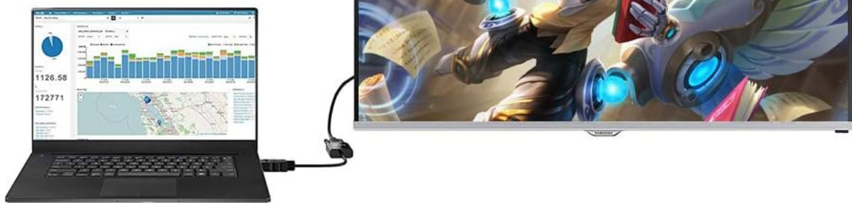
Image 4.1: Illustrations of Mirror Mode, where the laptop screen is duplicated on an external monitor, and Extend Mode, where the external monitor provides additional desktop space.
