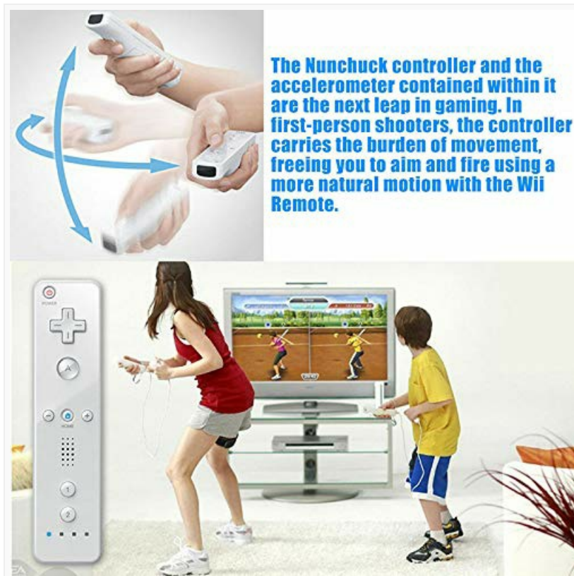
Figure 4: The Nunchuck controller's accelerometer detects movement, enhancing first-person shooter games by allowing natural aiming and firing.
