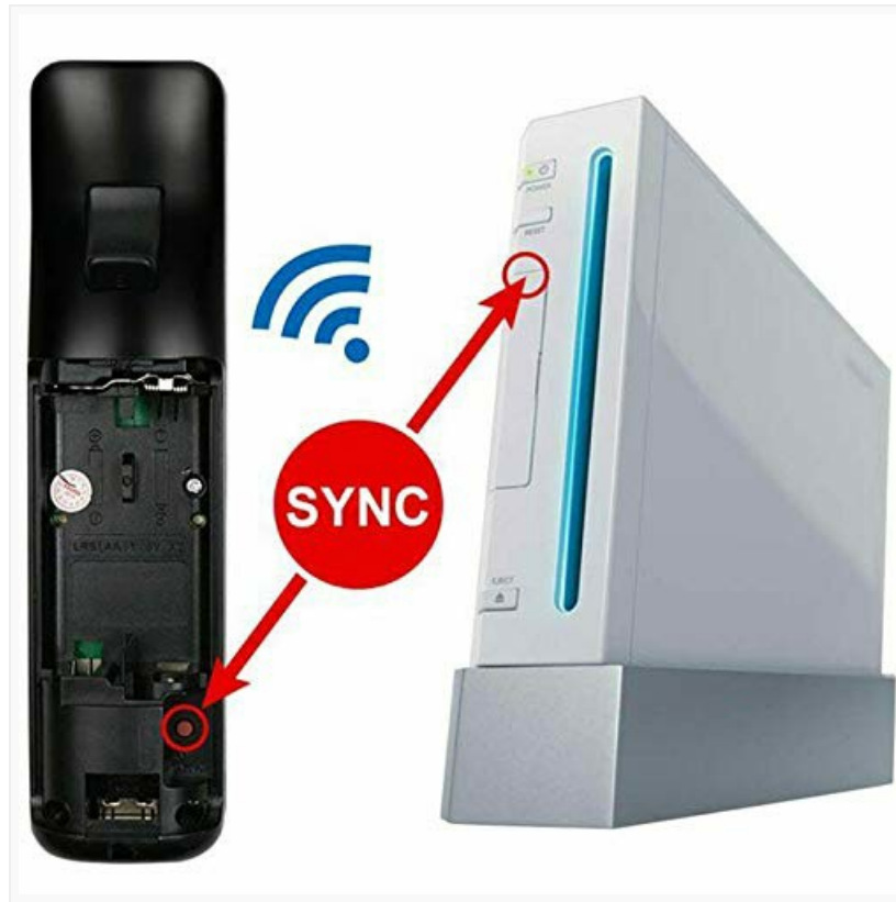
Figure 1: Location of the SYNC button on the remote and console for pairing. The remote shown is black, but the process is identical for the Sky Blue model.
