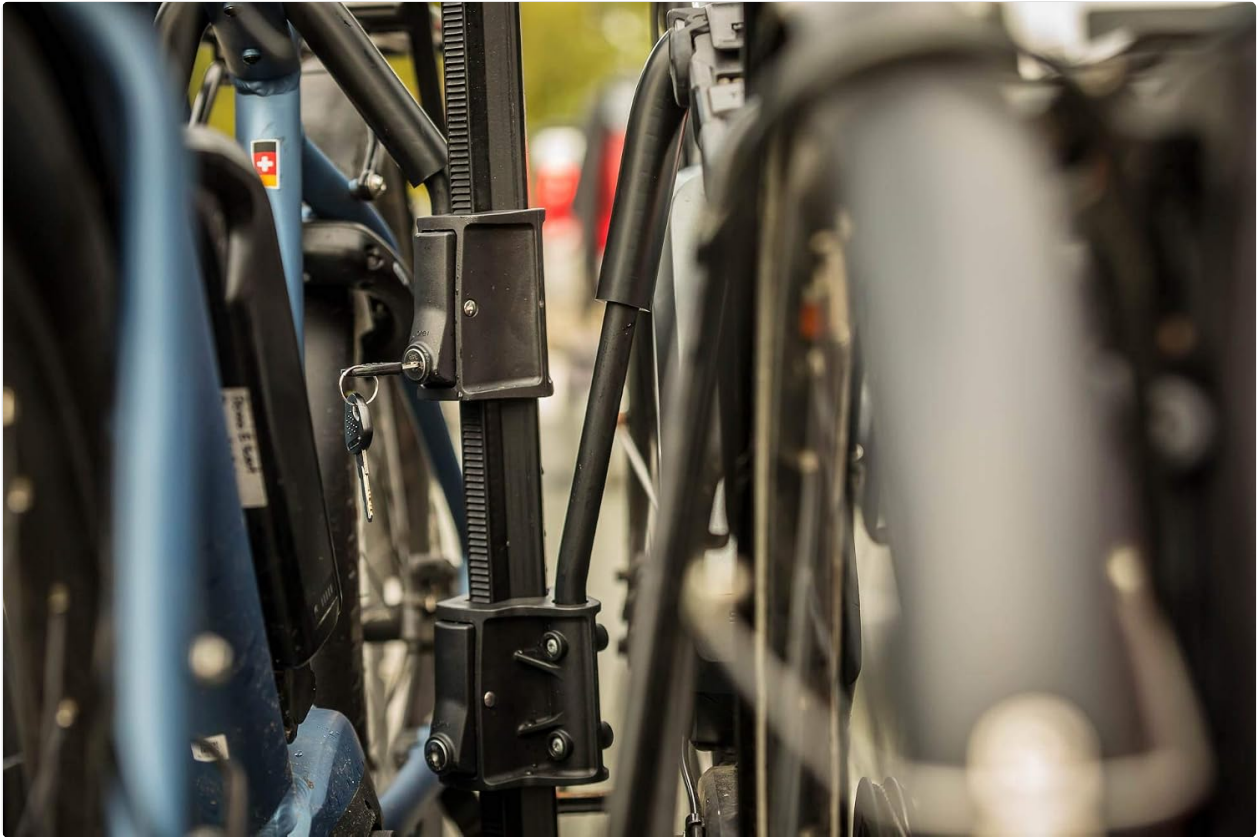
Figure 4: Detail of the locking ratchet hook for securing bike frames.
