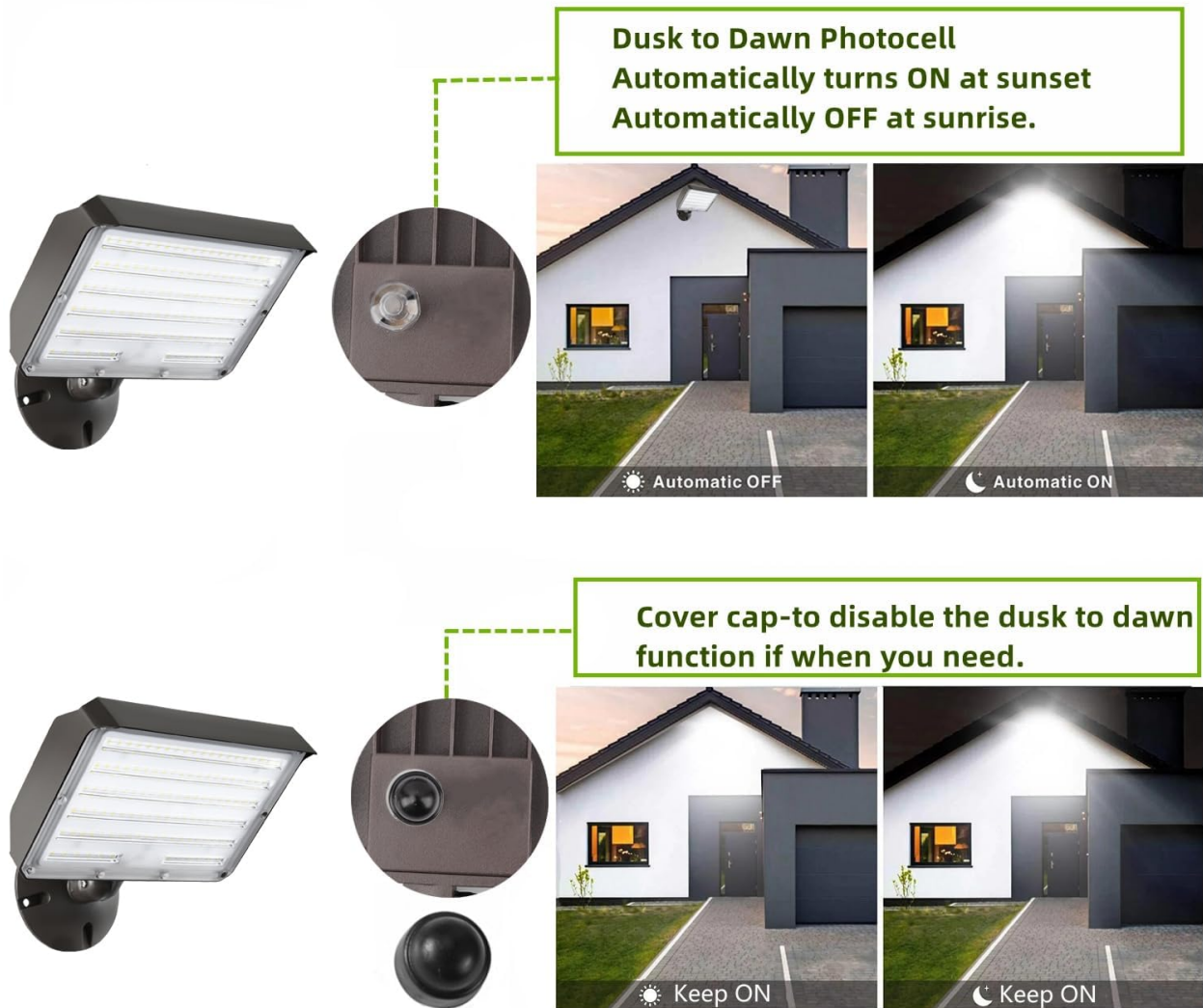
Image 7.1: Dusk to Dawn photocell operation and manual override.
