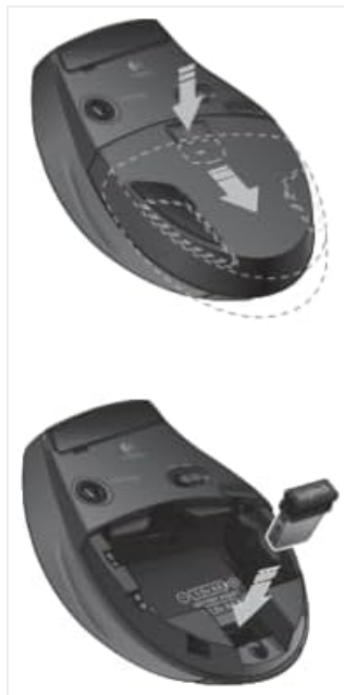
Figure 3: Steps for installing or replacing batteries in the M705 mouse.
