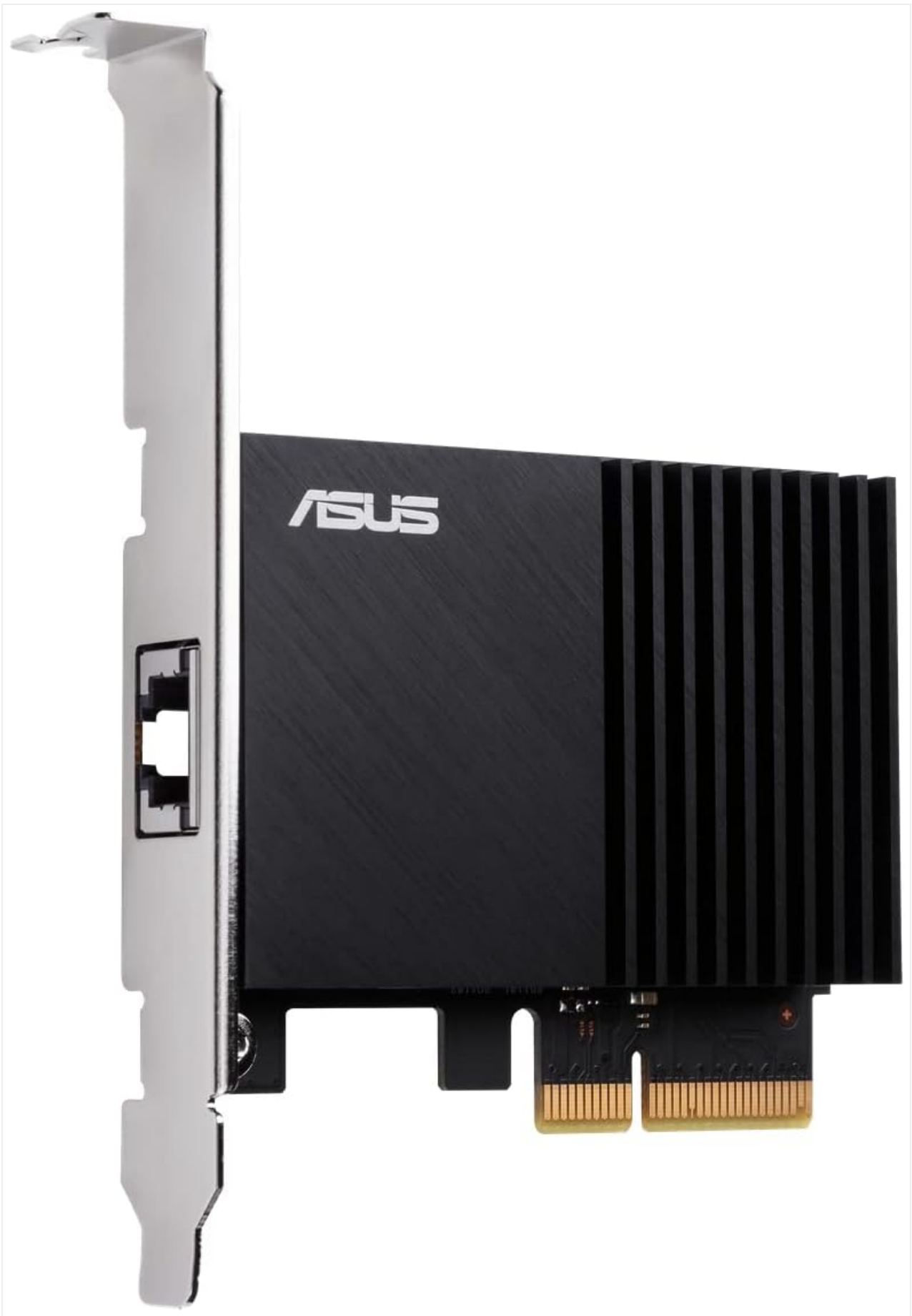
Image: The ASUS HYPER 10G LAN card, an accessory included with the motherboard.
