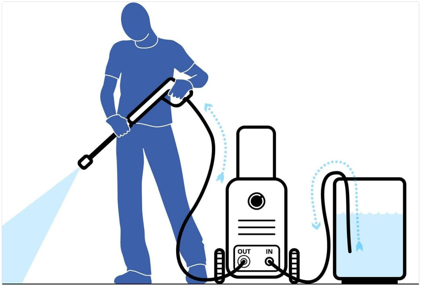
Figure 4.2: Diagram showing the pressure washer drawing water from an external tank using the self-priming function.
