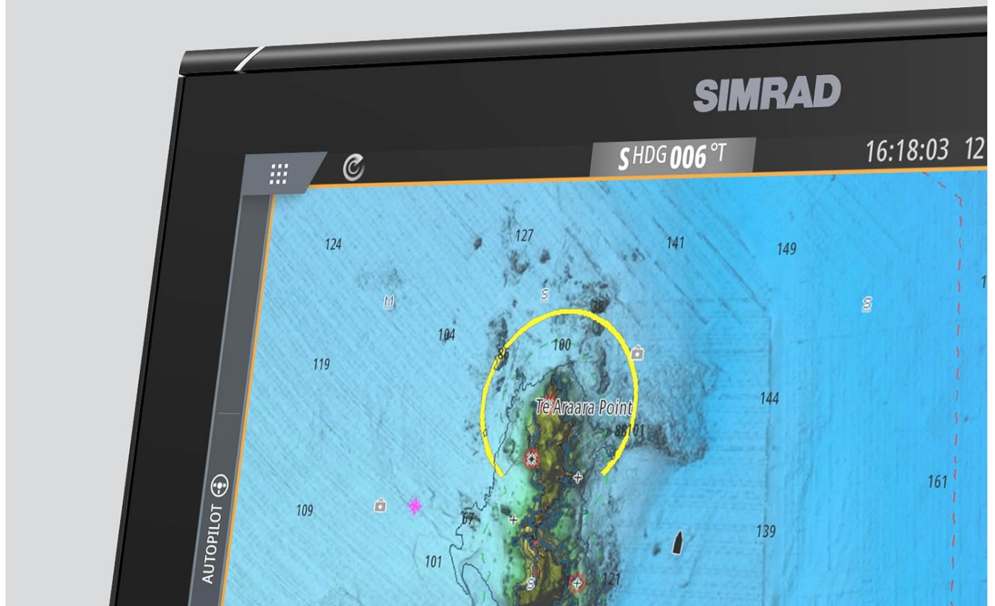
Figure 5: Chartplotter view on Simrad NSS12 Evo3S. This image shows the Simrad NSS12 Evo3S display in chartplotter mode, presenting a detailed navigational map. The screen illustrates depth contours, landmasses, and a highlighted area around 'Telamara Point', indicating the unit's capability to display comprehensive cartography for safe and efficient navigation.
