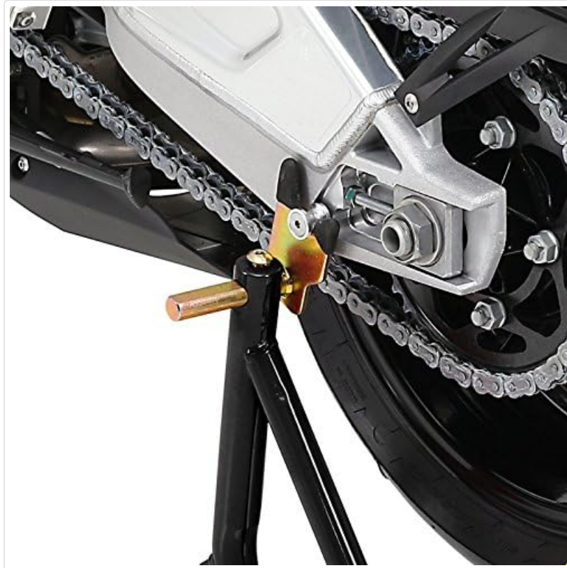
Figure 4: Close-up view of the rear stand's V-support engaging with a motorcycle's swingarm bobbin. This detail highlights the secure connection point.
