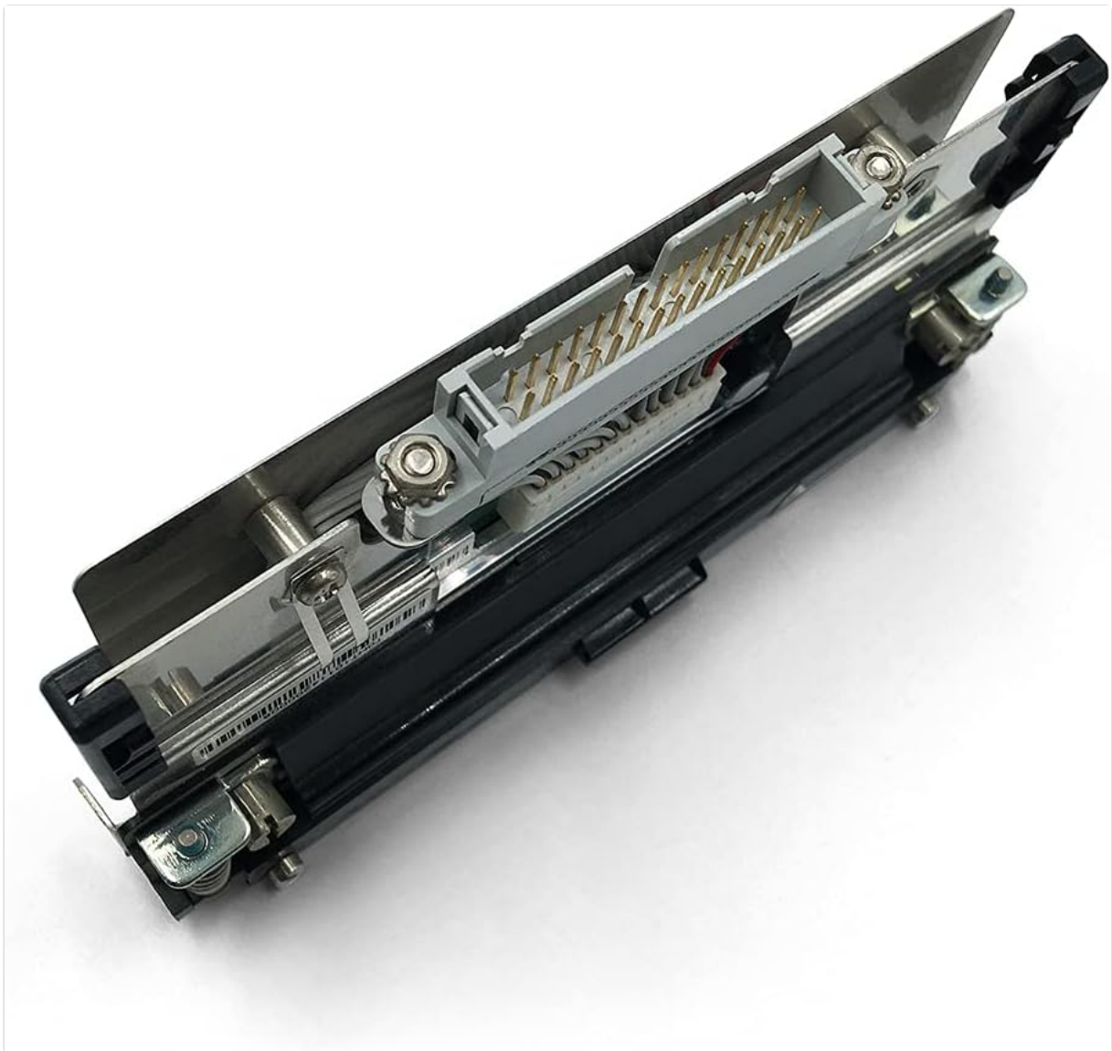
Figure 7.1: Bottom view of the printhead, displaying the array of electrical contacts. These contacts facilitate communication and power delivery from the printer to the printhead.
