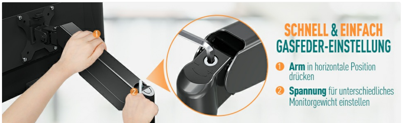
Figure 5: Gas Spring Tension Adjustment. Use an Allen key to adjust the tension screw. Turn clockwise for lighter monitors (decrease tension), counter-clockwise for heavier monitors (increase tension).
