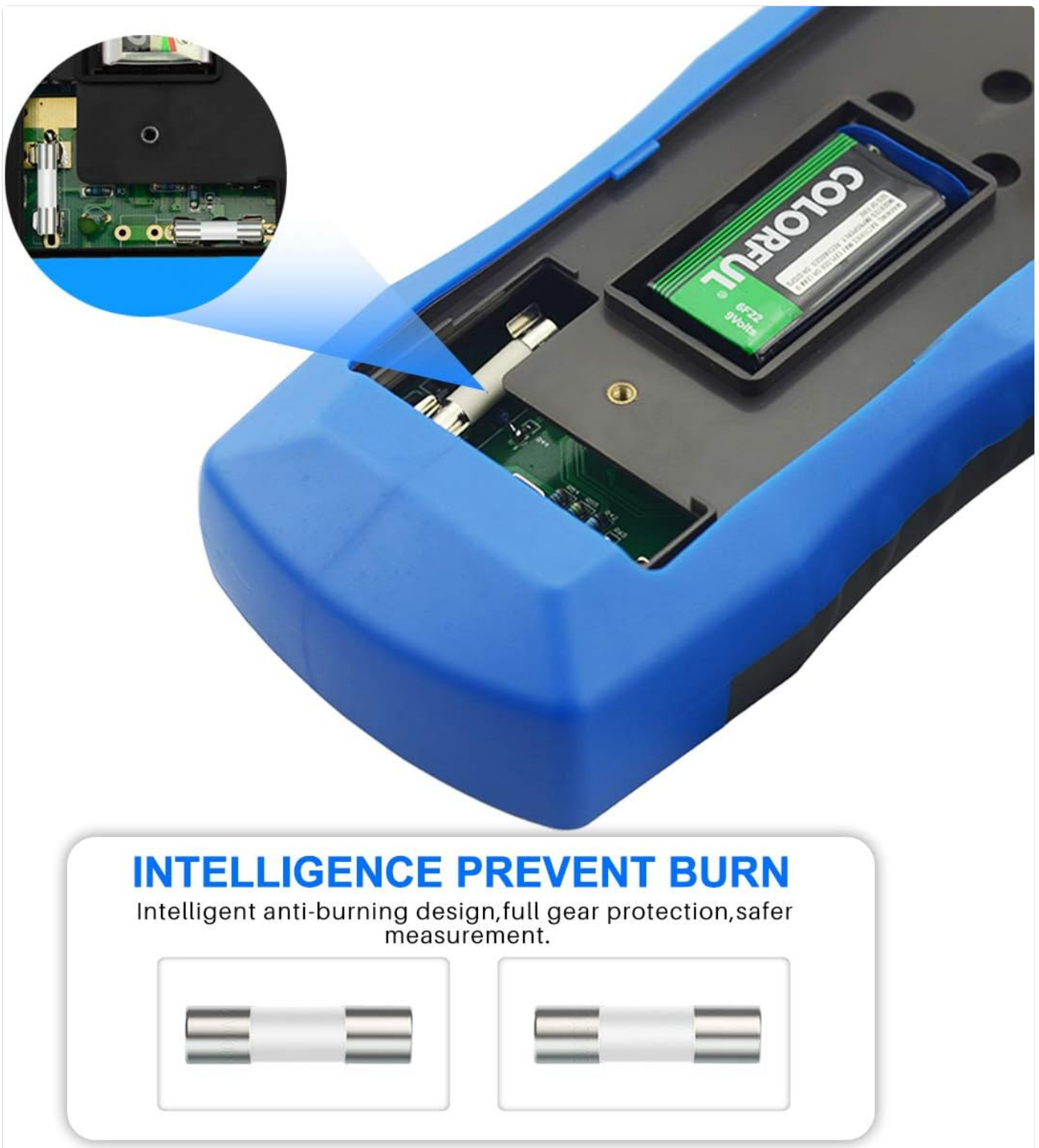
Image: The internal view of the Infurider YF-770N multimeter, showing the battery compartment with a 9V battery installed and the fuse location. This illustrates the 'Intelligence Prevent Burn' feature with full gear protection for safer measurements.
