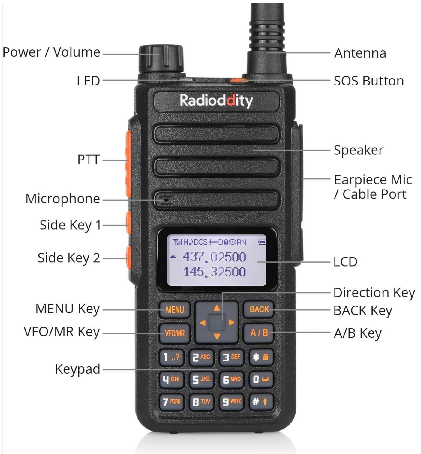
Image: A detailed diagram labeling the various components of the Radioddity GA-510, including Power/Volume knob, Antenna, LED indicator, SOS Button, PTT (Push-to-Talk) button, Speaker, Earpiece Mic/Cable Port, Microphone, Side Key 1, Side Key 2, LCD screen, Direction Key, MENU Key, BACK Key, VFO/MR Key, A/B Key, and Keypad.
