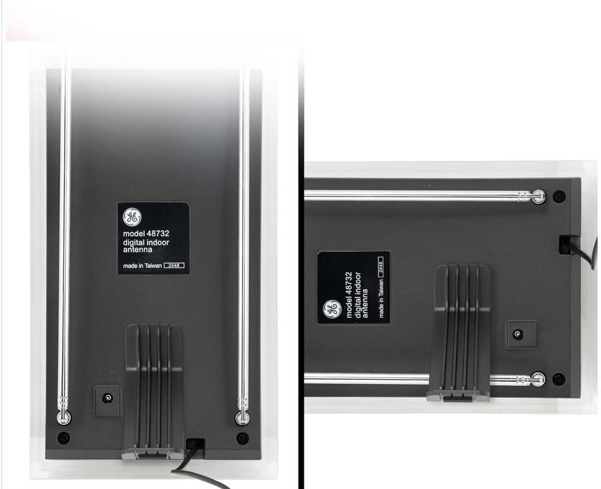
Image: The back of the antenna showing the adjustable stand, allowing for both vertical and horizontal positioning to suit different setups.
