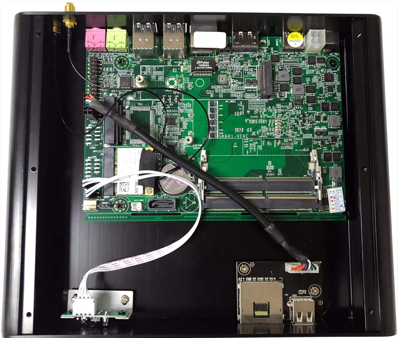
Image: An internal view of the KINGDEL NC860 Mini PC, displaying the motherboard, RAM modules, and M.2 SSD slot.
