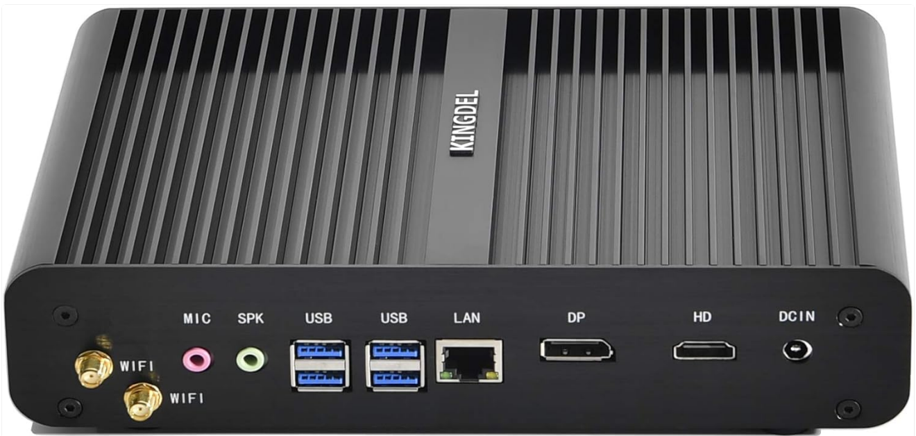
Image: Rear view of the KINGDEL NC860 Mini PC, displaying Wi-Fi antenna connectors, microphone and speaker jacks, two USB 3.0 ports, two USB 2.0 ports, a Gigabit LAN port, DisplayPort (DP), HD Port, and DC IN power input.
