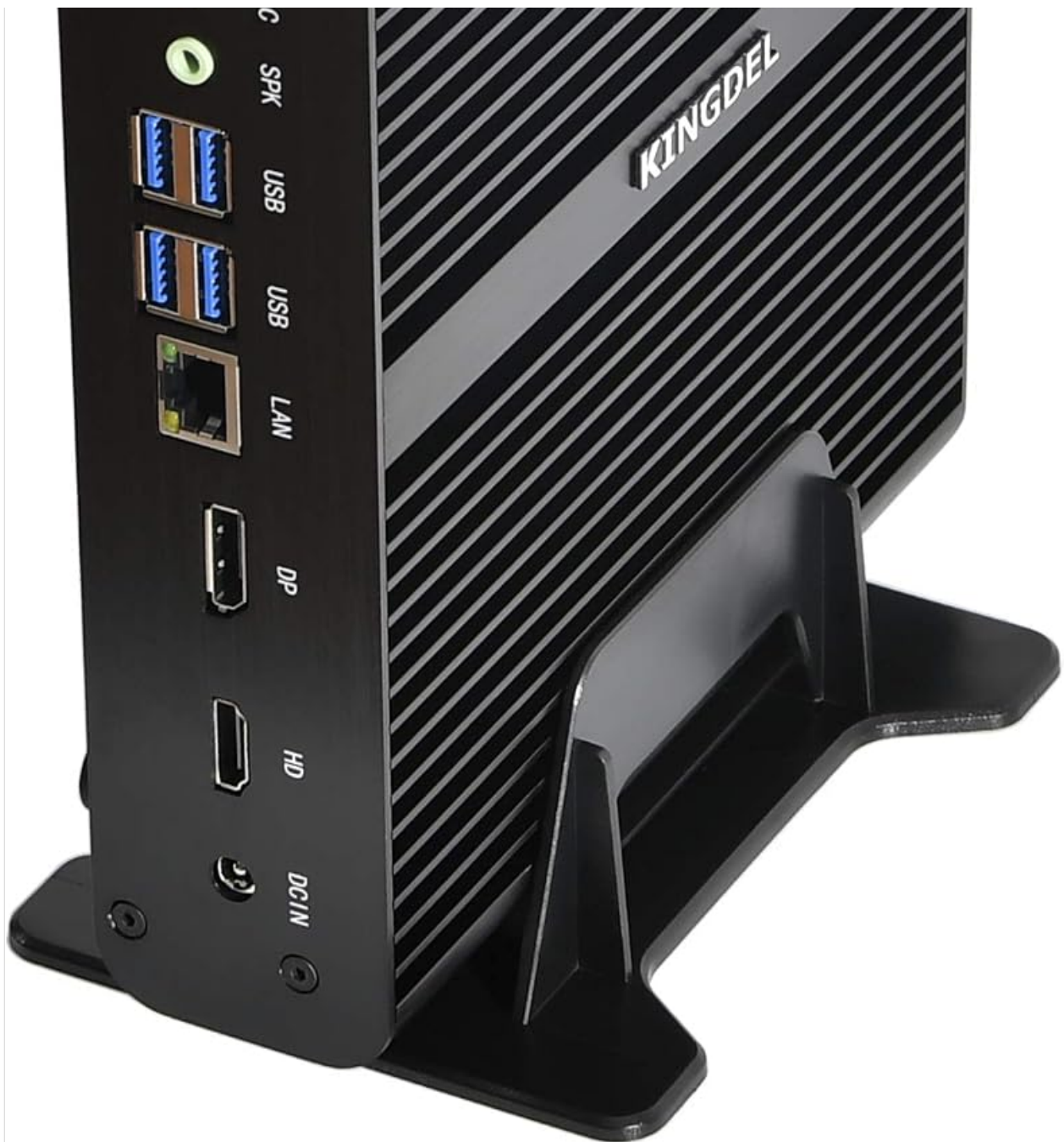
Image: The KINGDEL NC860 Mini PC positioned vertically in its included stand, showcasing the rear ports and Wi-Fi antennas.
