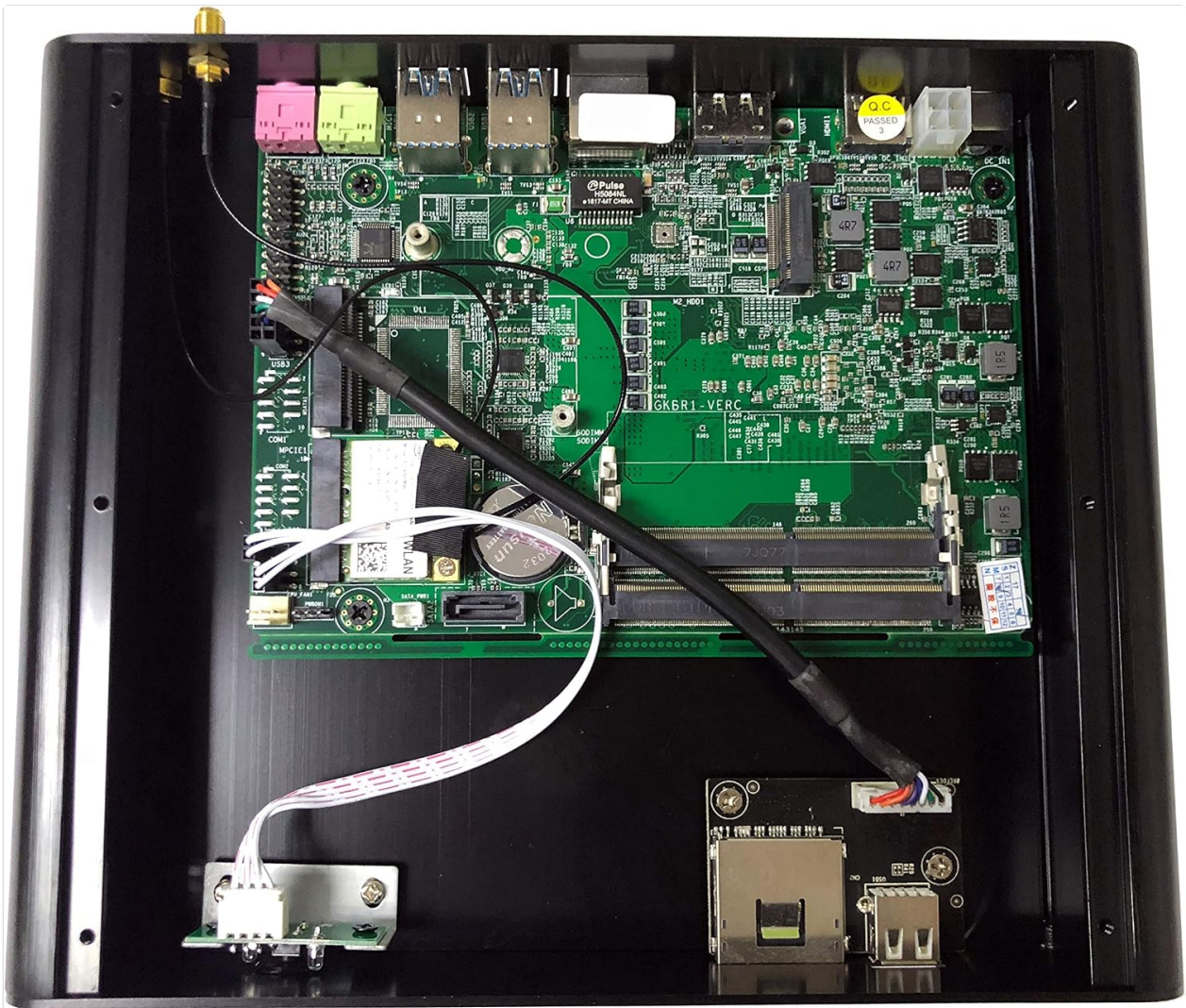
Image: An internal view of the KINGDEL NC860 Mini PC, showing the motherboard, RAM slots, M.2 NVMe SSD slot, and internal cabling.
