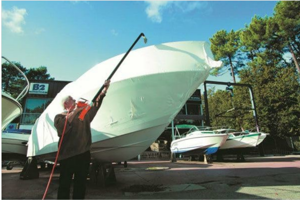
Image: A person demonstrating the use of a Ripack heat gun with an extension to apply shrink wrap to a large boat, highlighting the extended reach capability.
