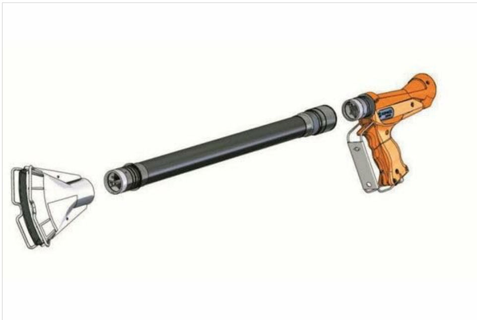
Image: Exploded view showing the heat gun, extension tube, and heat diffuser (nozzle) separated, illustrating how they connect. This diagram helps visualize the assembly process.
