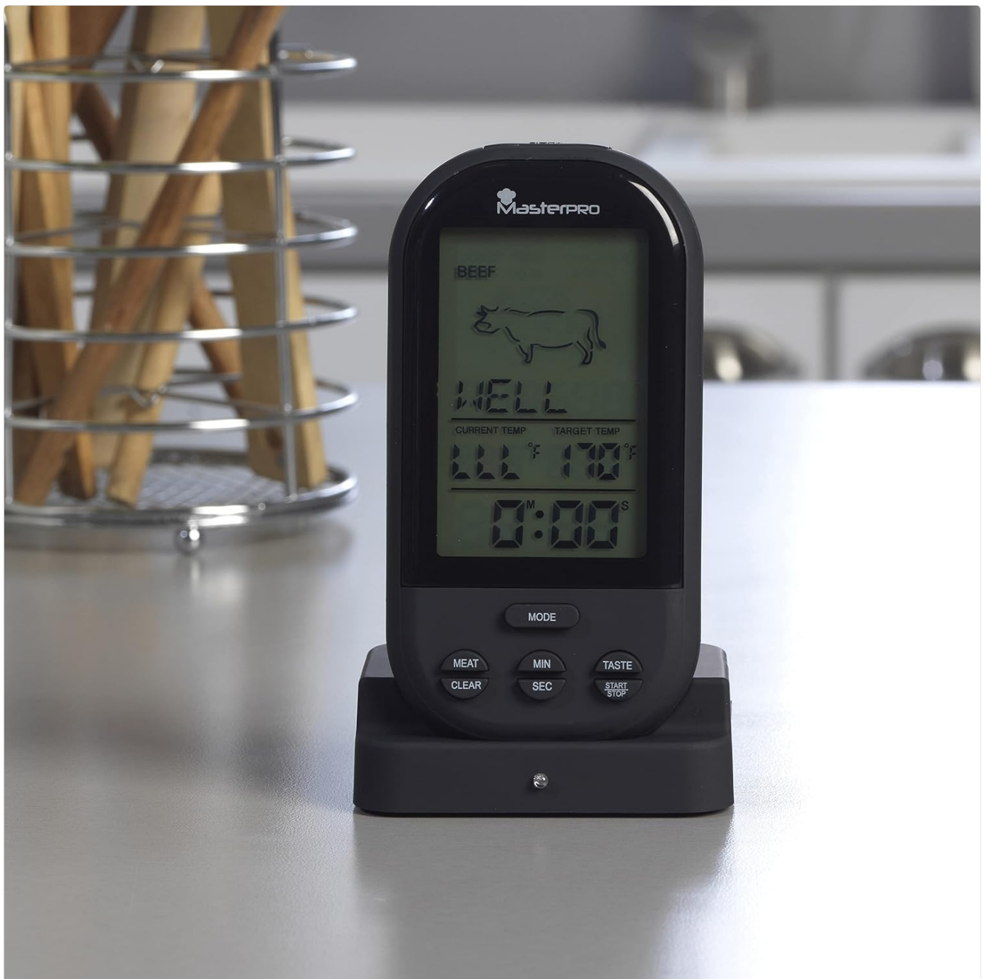
Figure 6.1: Example of "LLL" error display.
