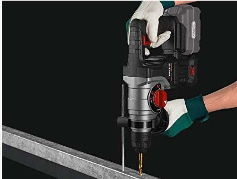
Figure 5.1: The rotary hammer drill being used in drilling mode on a metal beam. This demonstrates the tool's capability for precise drilling without impact, ideal for materials like metal or wood.
