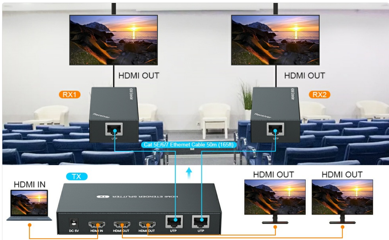
Figure 4.2: This diagram highlights the Power Over Cable (POC) feature, indicating that only the transmitter unit requires a power adapter, simplifying wiring for the receiver units.
