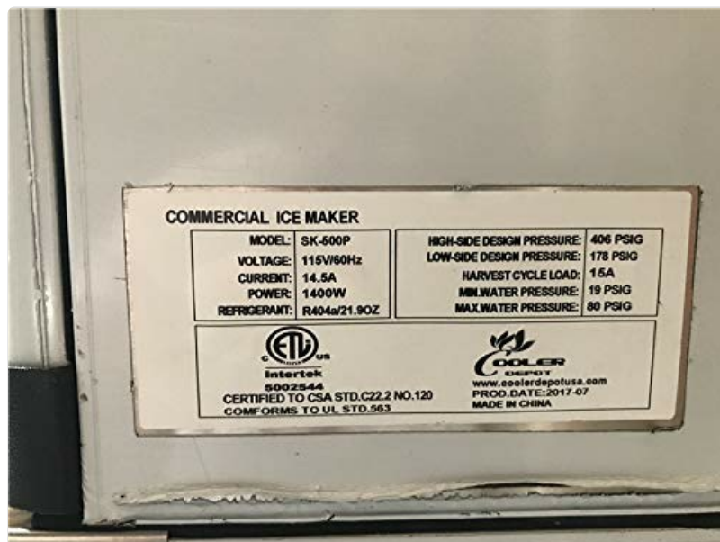
Image 7.2: Product specification label, showing model SK-500P, voltage, current, power, refrigerant, and pressure ratings.
