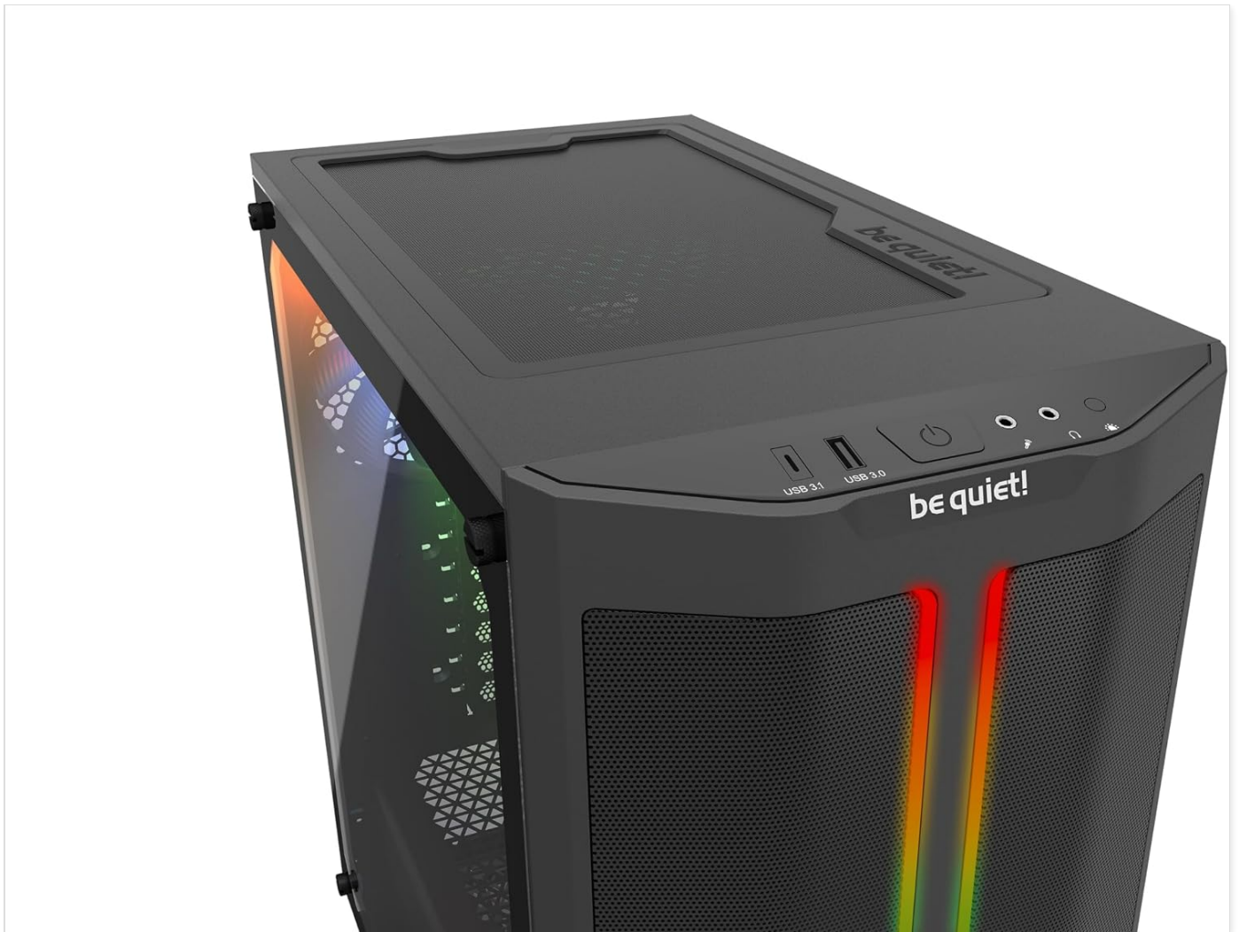
Figure 8: Close-up of the top I/O panel, featuring USB 3.1 Type-C, USB 3.0 ports, audio jacks, and the ARGB control button.
