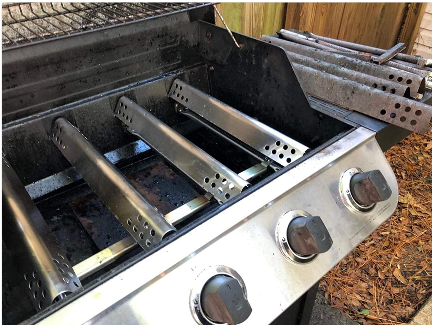
Image 7: An alternative angle showing the installed heat plates and burner tubes, providing a comprehensive view of the setup.
