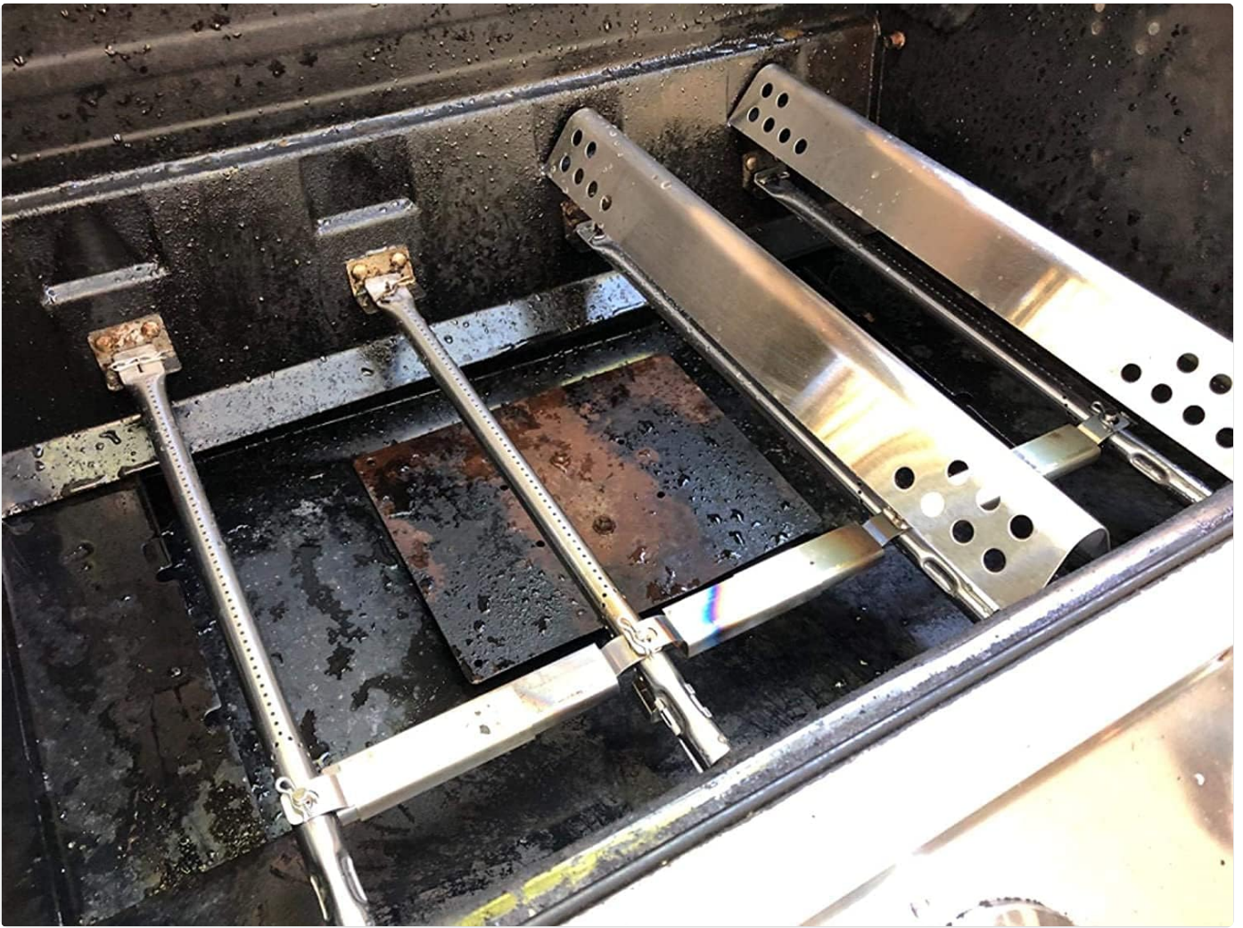
Image 6: Close-up view of the newly installed heat plates and burner tubes within the grill, showing proper alignment.
