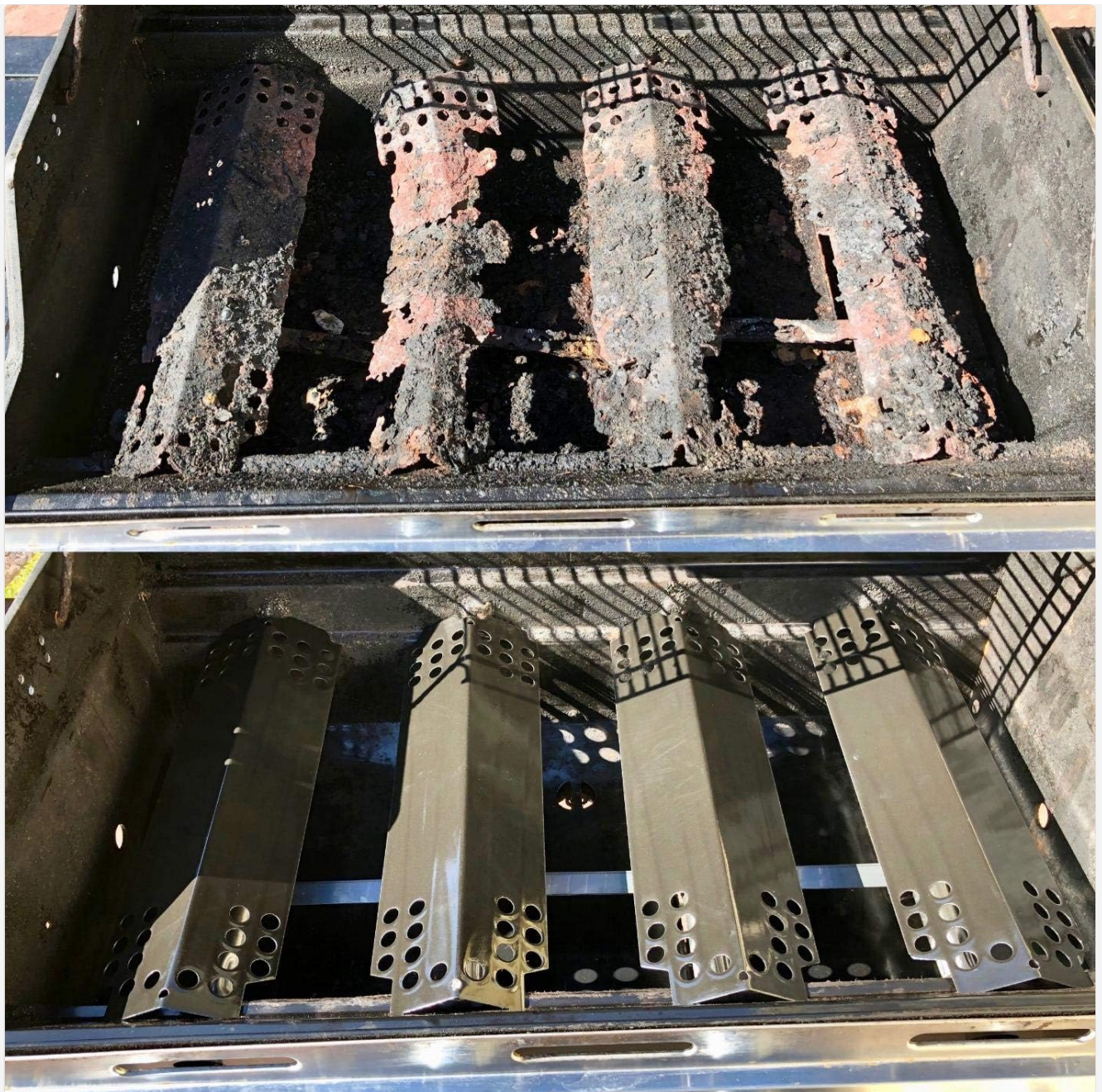
Image 5.2: Comparison of old (top) and new (bottom) heat plate tent shield installation.
