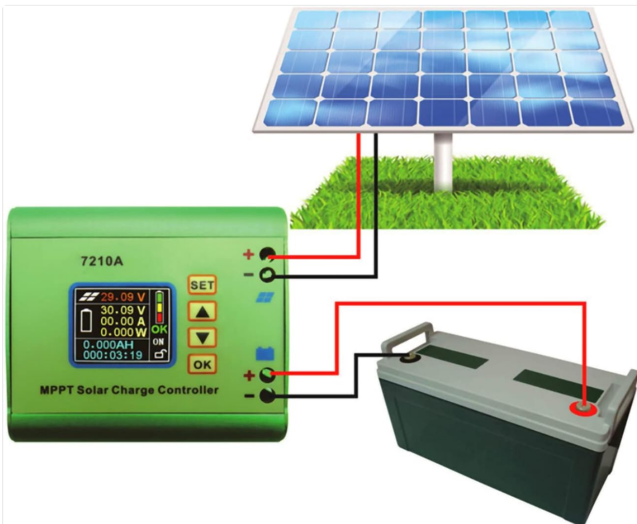
Figure 4: Wiring diagram for connecting the solar panel and battery to the MPT-7210A controller. Connect battery first, then solar panel.
