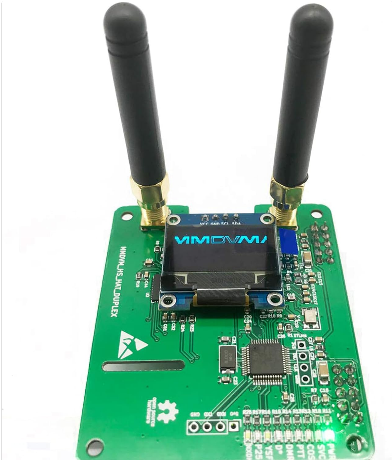
Figure 4: A detailed view of the MMDVM Duplex Hotspot Module, highlighting the 0.96-inch OLED display and the array of status LEDs (PWR, SVC, COS, PTT, DMR, YSF, P25, NXDN).
