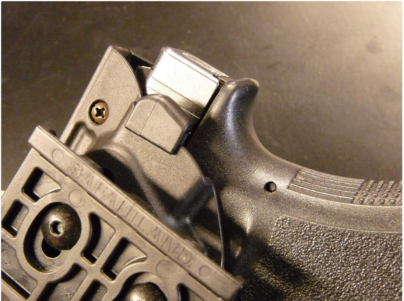
Close-up of the Automatic Locking System (ALS) mechanism inside the holster.
