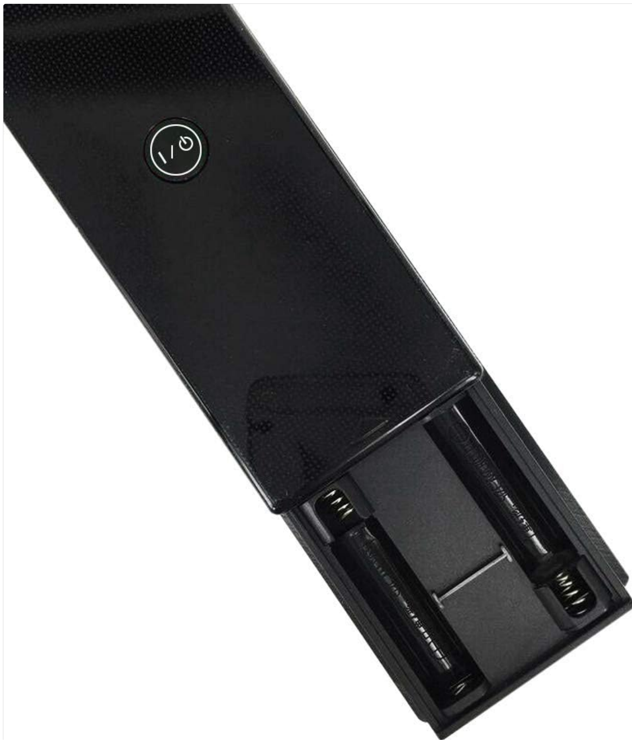
Image 2.1: View of the remote control with the battery compartment open, showing the slots for two AAA batteries.
