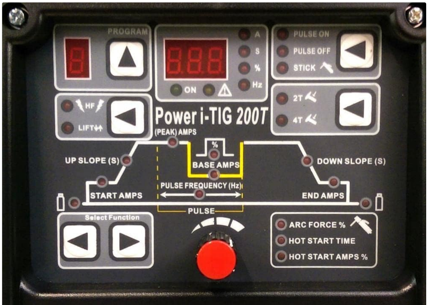
Image: Detailed view of the Poweri-TIG 200T control panel, showing digital displays for amperage, pulse settings, and various control buttons for TIG and Stick welding modes.
