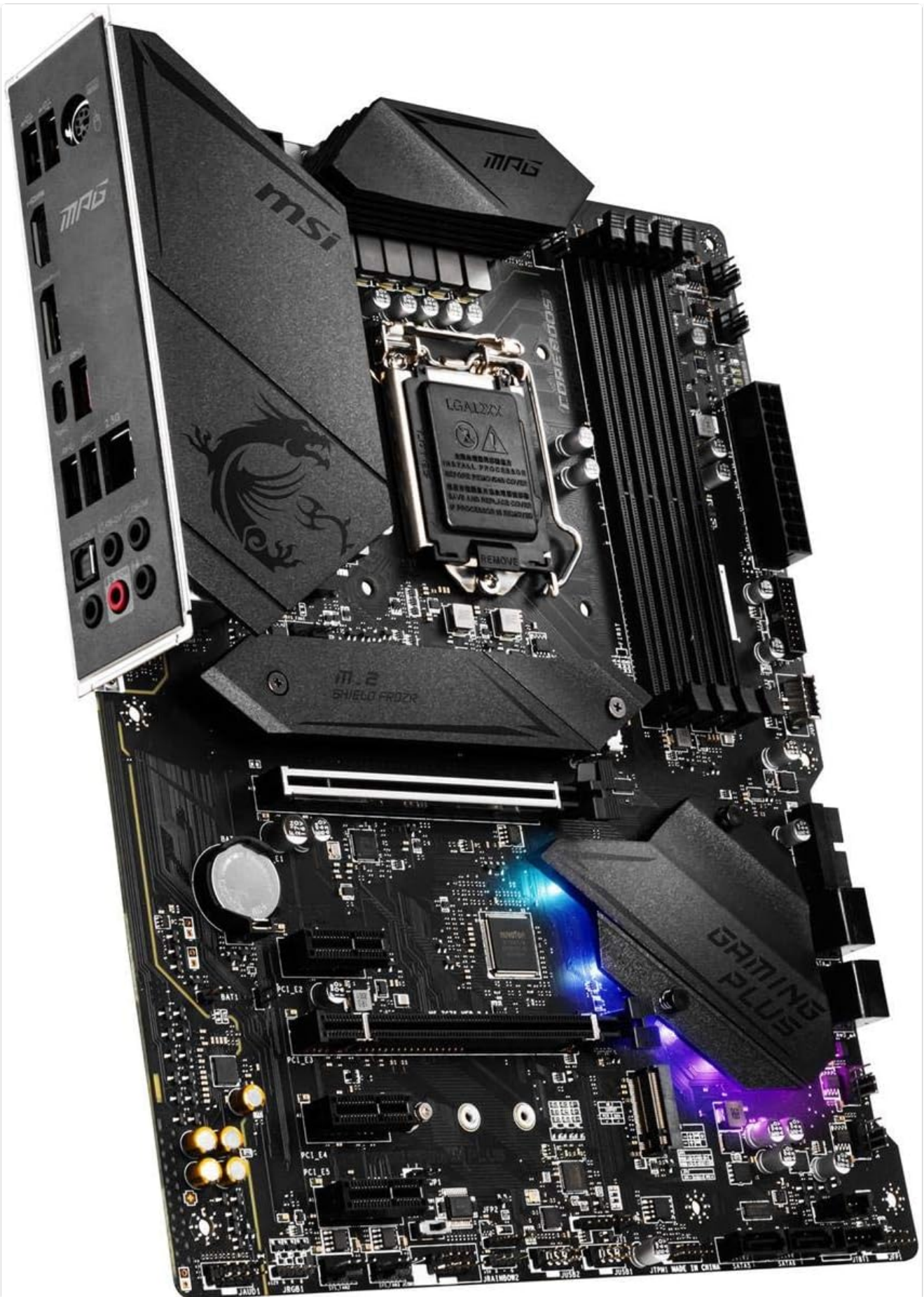
Image: An angled view of the MSI MPG Z490 Gaming Plus motherboard, showcasing the heatsinks, I/O shield, and PCIe slots.
