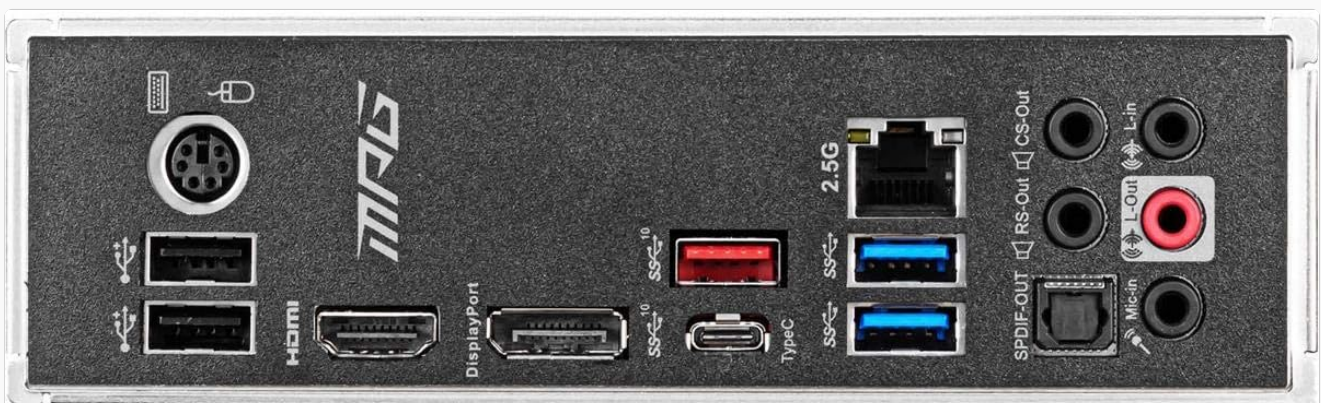
Image: A close-up view of the rear I/O panel of the MSI MPG Z490 Gaming Plus motherboard, showing ports for USB, HDMI, DisplayPort, LAN, and audio.
