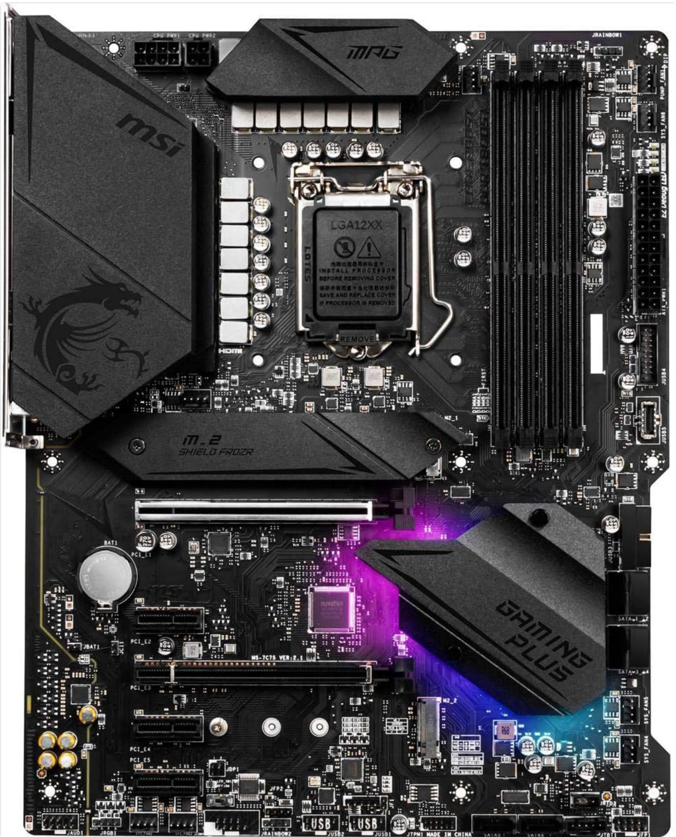
Image: A top-down view of the MSI MPG Z490 Gaming Plus motherboard, highlighting the CPU socket, RAM slots, M.2 slots, and various headers.
