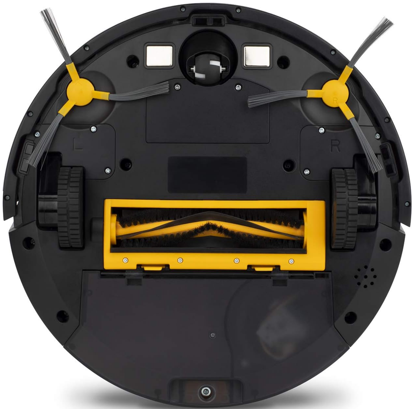
Image 2.2: Underside view of the H.Koenig SWRC120, showing the main brush, side brushes, and wheels.
