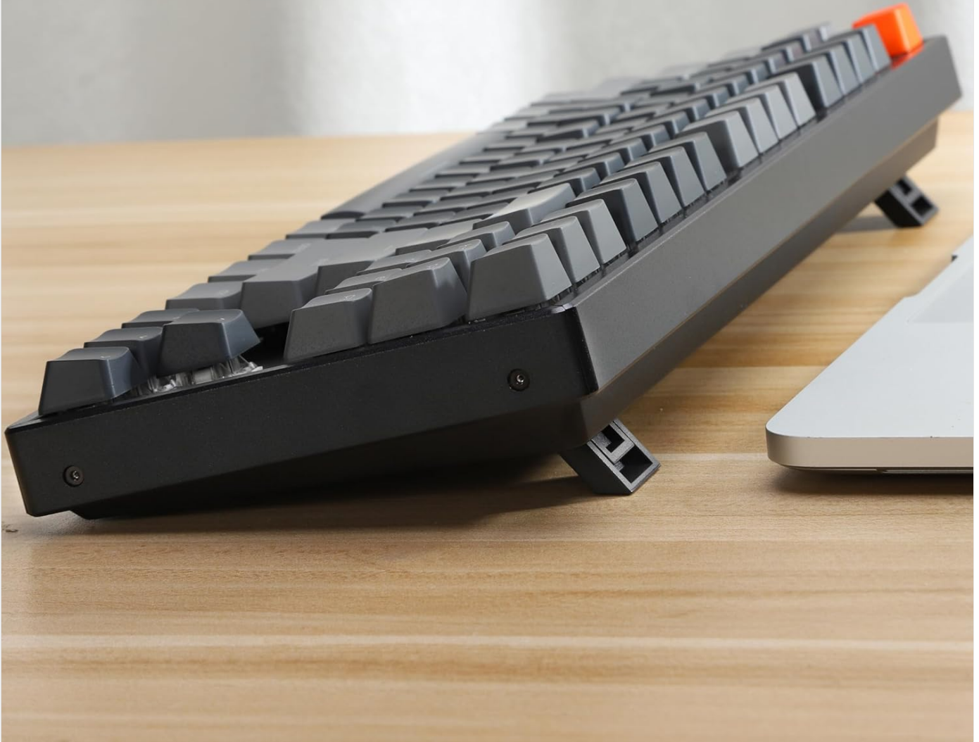
Image: A side view of the Keychron K8 keyboard, illustrating its two adjustable angled feet in an extended position.
